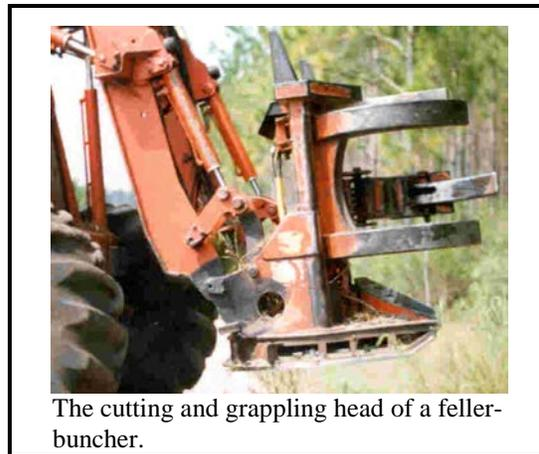
The cutting and grappling head of a feller-buncher.
